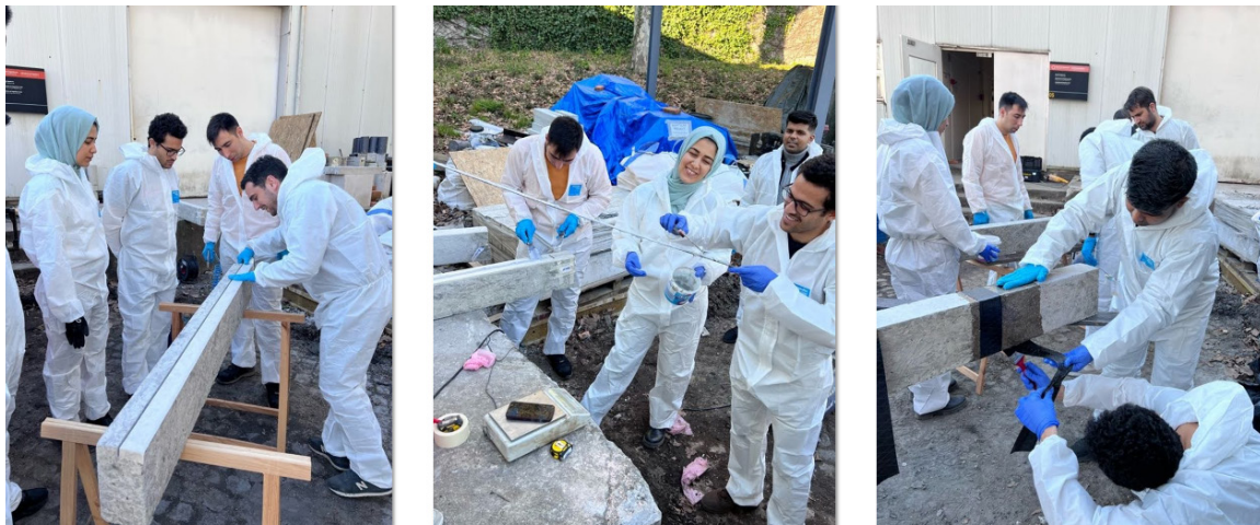
Figure 6. Strengthening of RC beams in the context of FRP++5.
