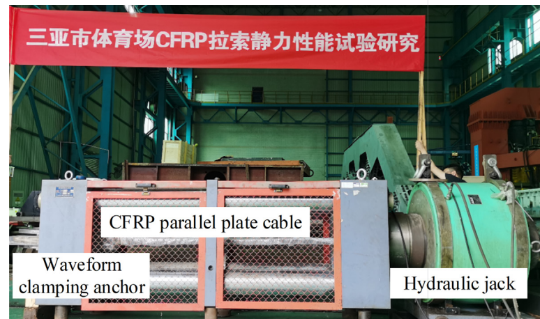
Figure 5. Test loading device.
