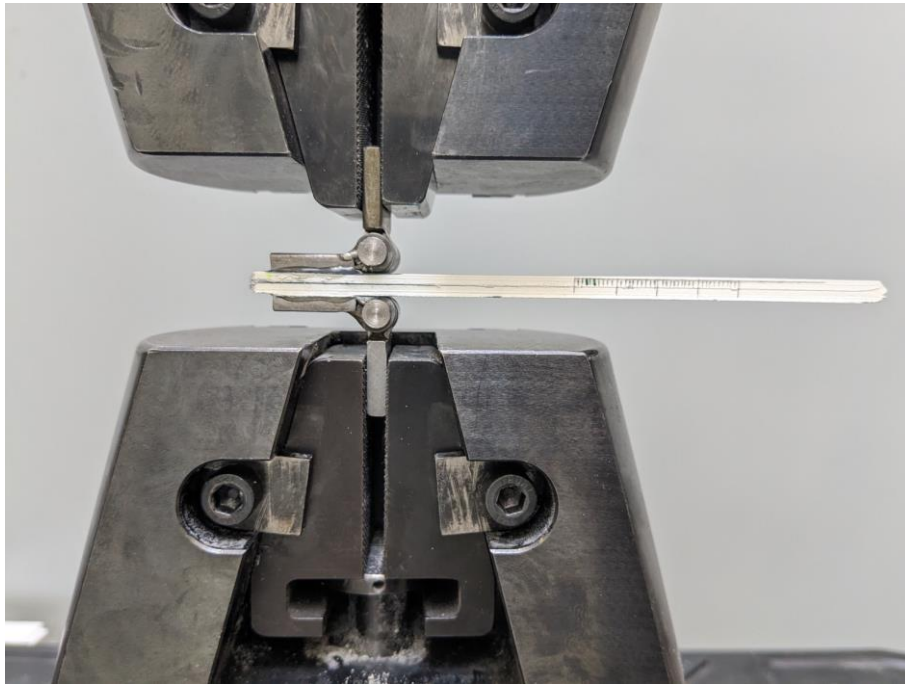
Figure 3.20: Setup of the DCB test.
