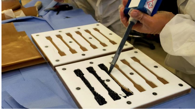
Figure 3.9: Application of the adhesive.
