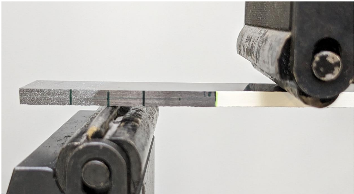
Figure 3.27: Compliance calibration markings on the ENF specimen.
